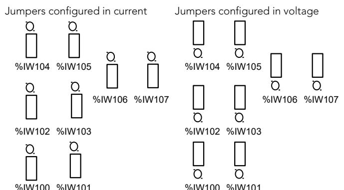
Value range from 0 to 10000 if configured in voltage and 0 to 20000 if configured in current
